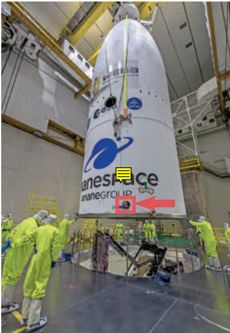
CCD area highlighted on Ariane 5 PLF ©ESA/CNES/Arianespace [highlights by the author]
